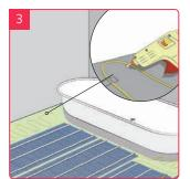
For irregular areas Remove the cable from the mesh, arrange and stick down the excess mesh
