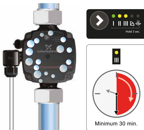
Fig. 7 Venting the pump
